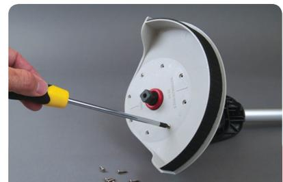
3. Attach the splash-guard bracket with the base plate screws. Start with any screw then insert the opposite one, tighten. Tighten the remaining six screws in the same manner.
