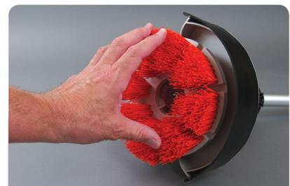
6. Twist-lock brush to the hub and reconnect the power supply.
