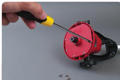
2. Remove the screws that hold the base plate to the motor housing without removing the base plate.
